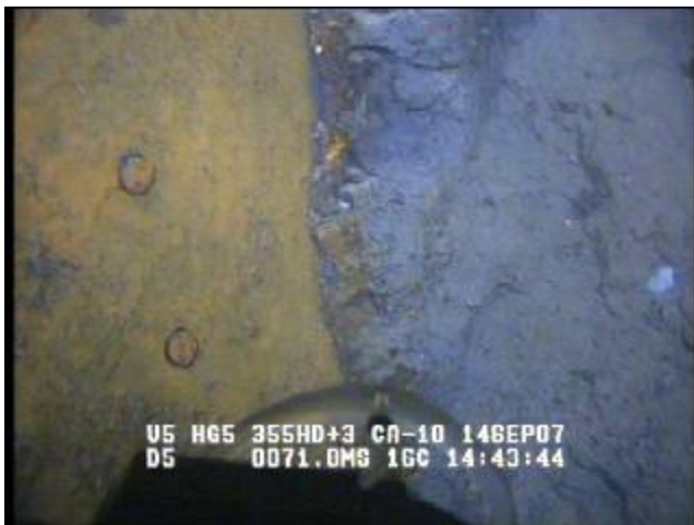
Figure 30. ‘Started’ rivets on portside saddle tank.
