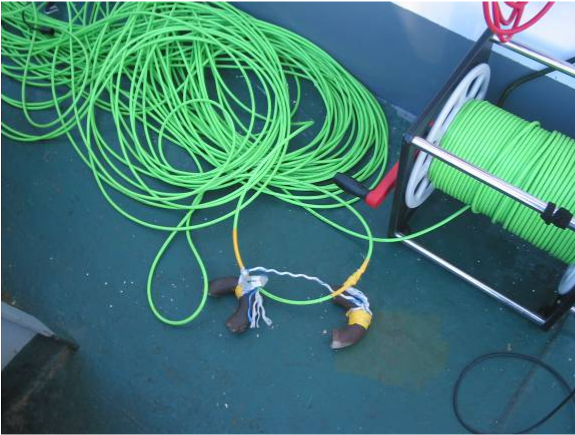
Figure 2. A pair of chain half links was used to carry the umbilical directly to the seabed. Video-based Survey Tasks Undertaken by the ROV
