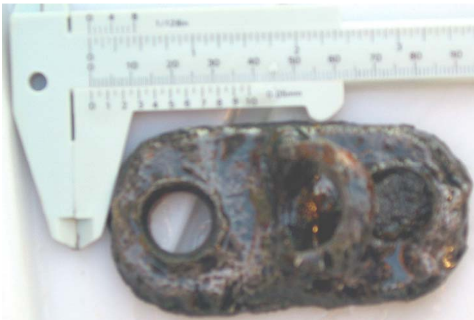
Figure 7: Details of the ring and sheared off bolt fitting from the side of the submarine
