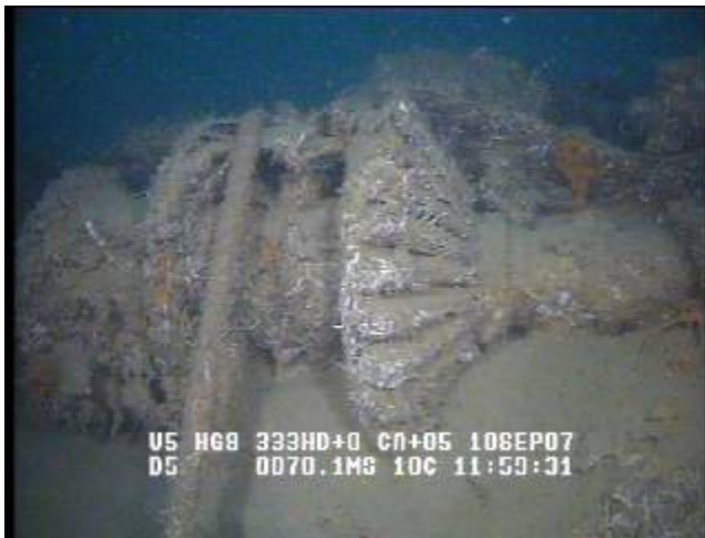
Figure 8. Anchor Winch, looking from the port side. The rope lying over is fishing debris.
