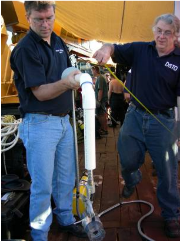
Figure 31. Showing the general arrangement of the drop camera with Mr Peter Graham DSTO ROV pilot left and Dr Roger Neill Task Overseer.
